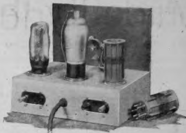
Eddystone All-World-Two receiver assembled from the kit of parts.
