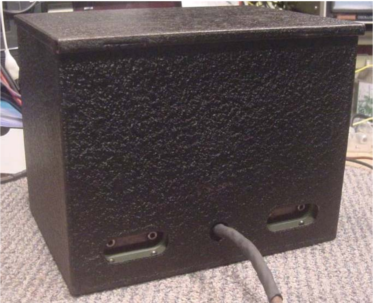
Rear view of the AW2 – the original power cord was reinforced with heat-shrink tubing at its point of entry through the case (it had become frayed at this point). The 'phones connect to the left hand sockets and the aerial and earth to the right hand ones
